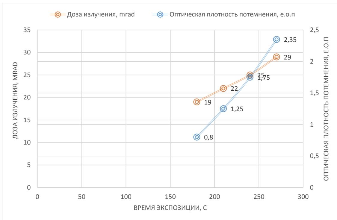
Figure 3.5 Dependence of darkening density and radiation dose on exposure time F8+RCF,
