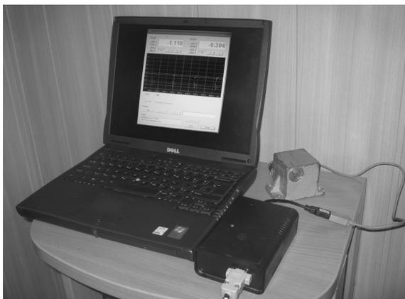
**Fig. 10.** The appearance of programme-production vibroanalyser complex prototype
