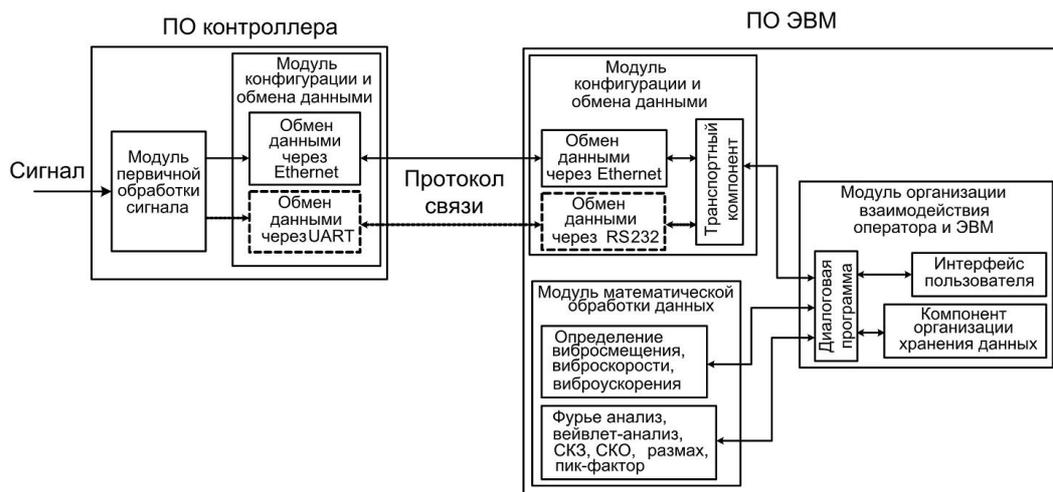
Fig. 8. Simplified structural diagram of the software
