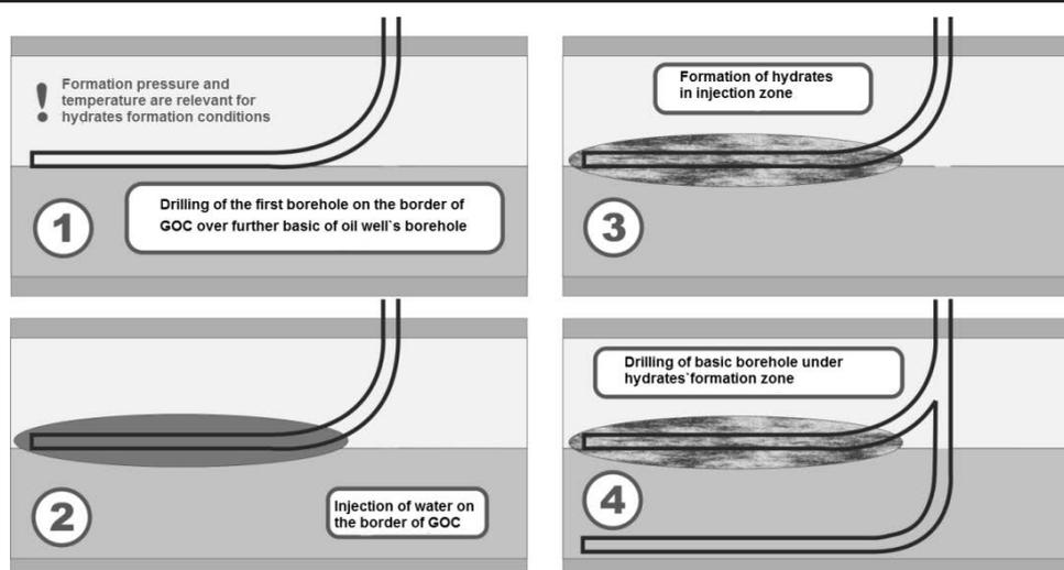
*Fig. Stage-by-stage process of formation of hydrates*
