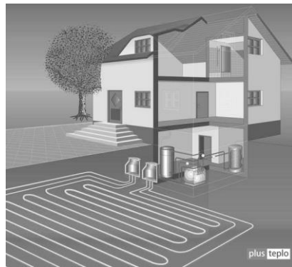
Figure 2 – Horizontal outer contour of the heat pump an apartment house
