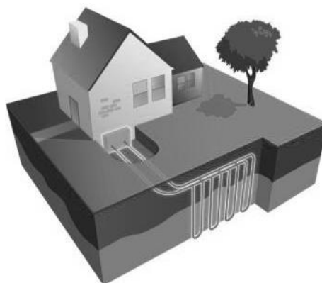
Figure 3 – The outer loop heat pump vertical type
