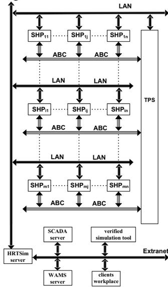
**Figure 2.** Structure of the HRTSim: SHP - specialized hybrid processors; LAN – local area network; TPS – three-phase switch; ABC – three-phase input/output of SHP
