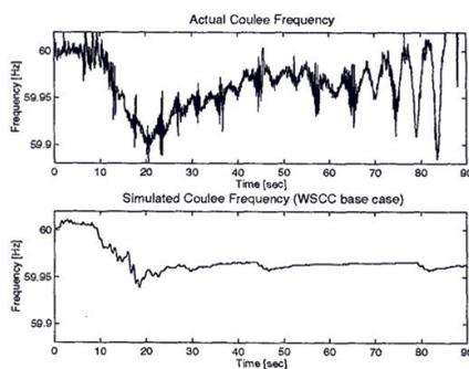
**Figure 1.** Grand Coulee unit 20 frequency – recorder and simulated using PMU data base
