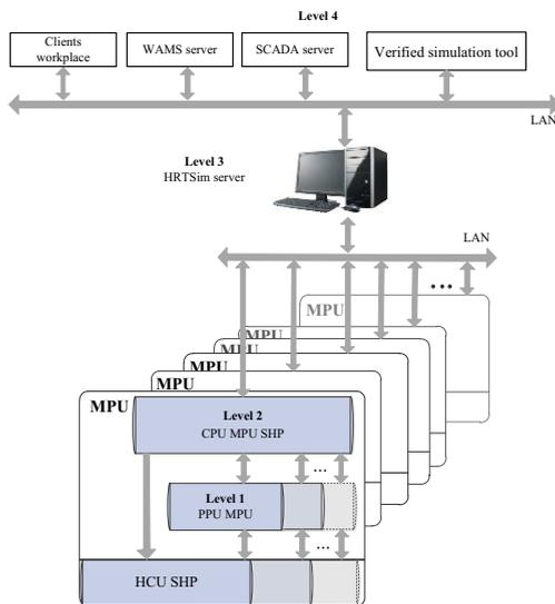
**Figure 3.** The structure of the multi-level information and control system: CPU – central processing unit, MPU – microprocessor unit, PPU – peripheral processor unit, HCU – hybrid coprocessor unit
