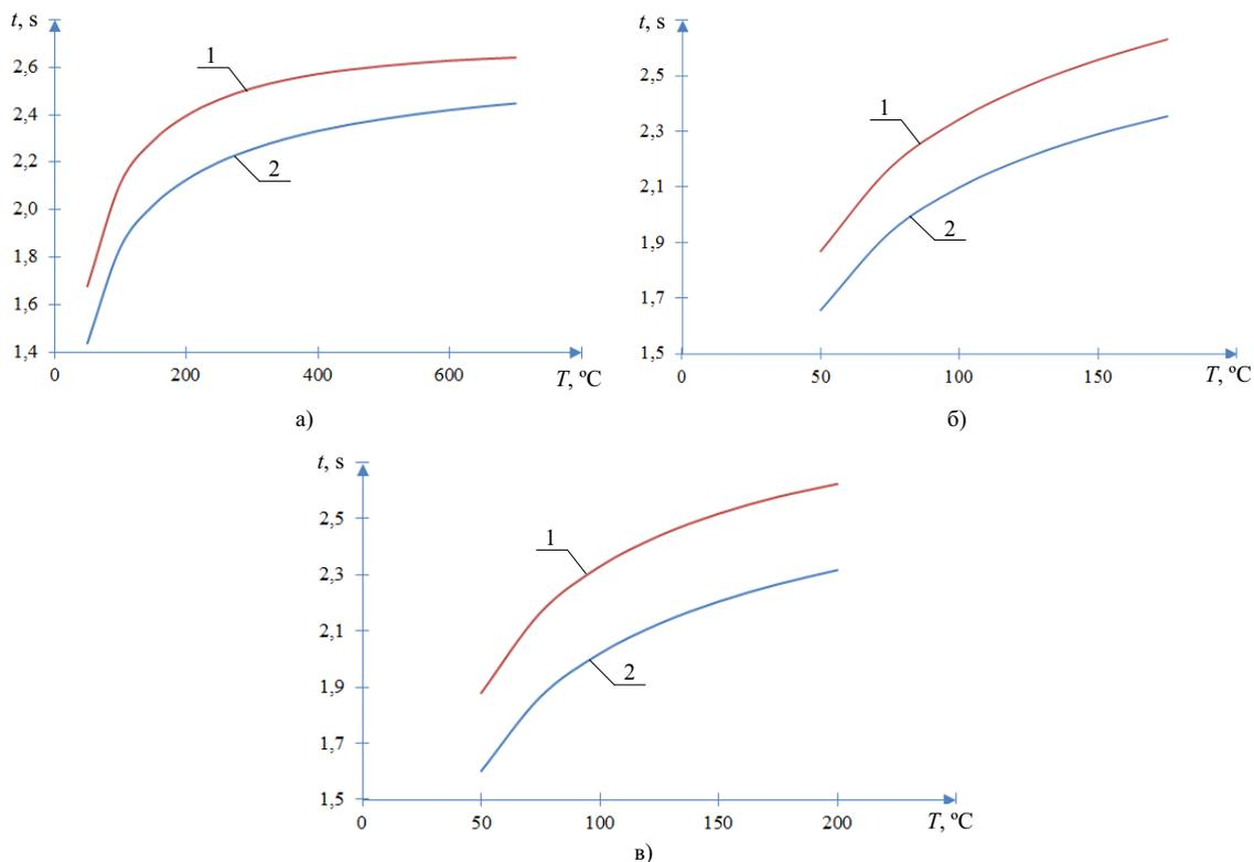
**Figure 2.** Dependence of necessary duration of heating up of TPS on the taken temperature: a – platinum RTD; – nickel RTD; in – copper RTD; 1 – the approximated heatphysical characteristics; 2 – constant heatphysical characteristics
