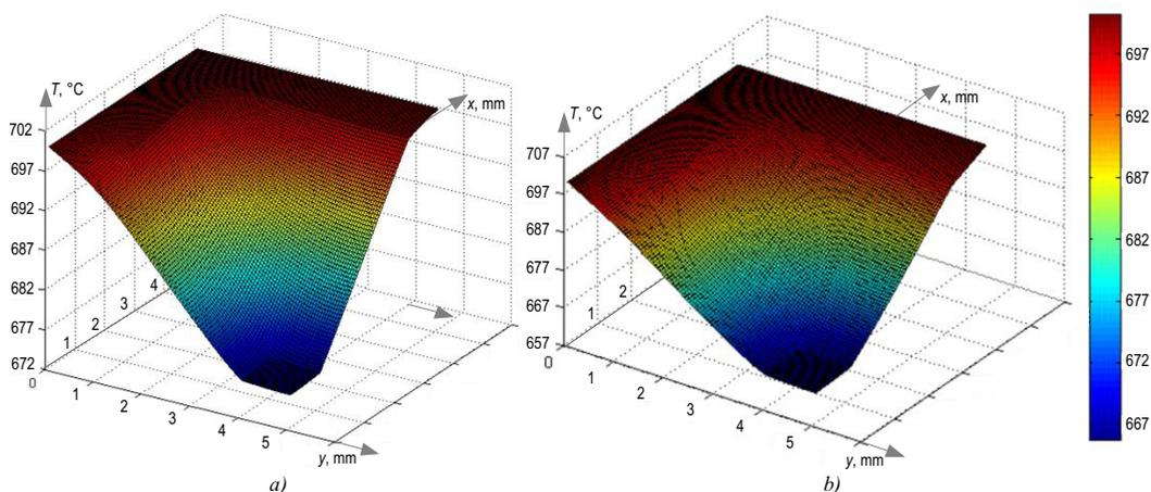
Figure 3. Temperature fields in a sensitive element of platinum RTD at measurement of temperature 700 zs, received by means of constants (1) and the approximated (2) and heatphysical characteristics
