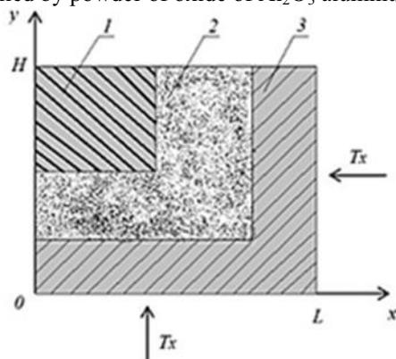
**Figure 1.** the Diagram of area of the solution of the task: 1 – sensitive element; 2 – isolation powder ( $Al_2O_3$ ); 3 – metal jacket (steel); H – height of a section of the RTD sensitive element; L – radius of the RTD sensitive element
