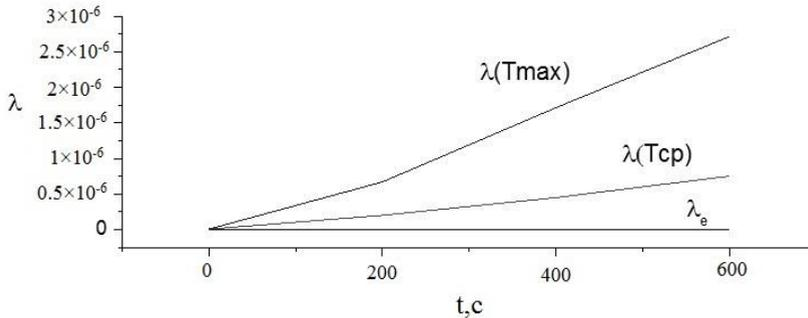
**Figure 4.** Failure rate of single-wire conductor at an ambient temperature  $T = 250\text{C}$ ,  $t = 600$  sec. ( $\lambda_e$  - multiplicative model ;  $\lambda(T_{av})$  - Arrhenius model (with  $T_{av}$ );  $\lambda(T_{max})$  - Arrhenius model (at  $T_{max}$ ).
