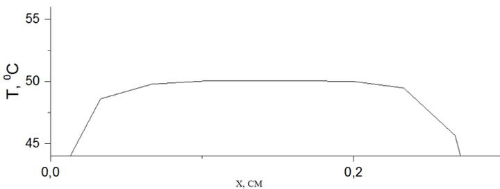
**Figure 3.** The temperature distribution on plate thickness in a timepoint  $t=15\text{sec}$  and amperage  $I=10\text{A}$ , the environment temperature is  $t=25^{\circ}\text{C}$
