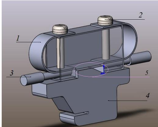
**Figure 1.** Contact connection with socket terminals: 1 – terminal block; 2 – screw ; 3 – conductor ; 4 – corps; 5 – section plate;
