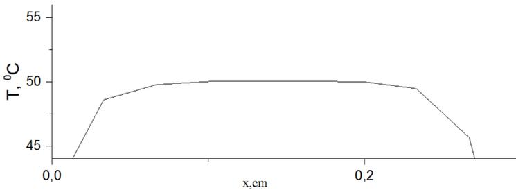
**Figure 2.** The temperature distribution on plate thickness in a timepoint  $t=15\text{sec}$  and amperage  $I=4.4\text{A}$ , the environment temperature is  $t=25^\circ\text{C}$
