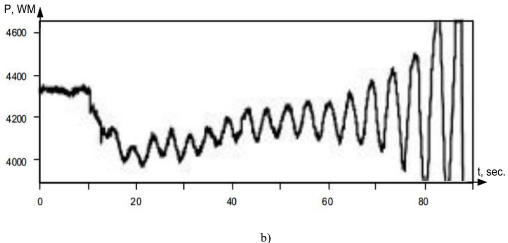
**Figure 1.** Oscillogram of the power flow obtained by digital models (a) and WAMS (b).
