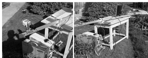
Fig. 4. Breadboard of TV stereo range finder
