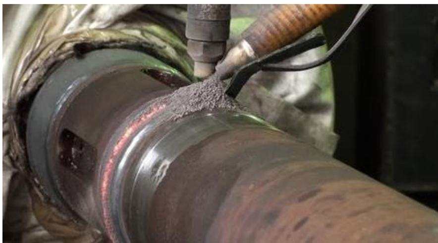
Image 1. Submerged-arc welding
