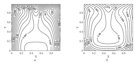
**Figure 5.** Fields temperature in the LNG storage tank: *a*) with the heat insulation on lower boundary (q = 0), *b*) with the heat flow on lower boundary  $(q = 0.05 \text{ W/m}^2)$ .
