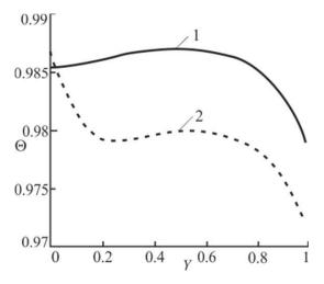
Figure 7. Temperature profile in the section X = 0.5,  $0 \le Y \le 1$ : 1) with the heat insulation on lower boundary (q = 0), 2) with the heat flow on lower boundary  $(q = 0.05 \text{ W/m}^2)$ .
