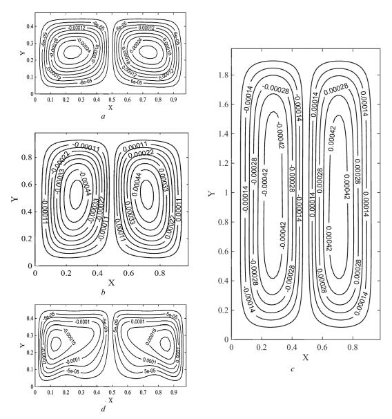
**Figure 2.** Contours of stream function in the storage tanks LNG with different geometric dimensions: a) l = 10 m, h = 5 m; b) l = 10 m, h = 10 m; c) l = 10 m, h = 20; d) l = 20 m, h = 10 m. The numerical values of coordinates and temperatures are given in a dimensionless form.
