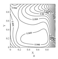
**Figure 8.** Fields of temperature with different heat flows on the left  $(q = 0.05 \text{ W/m}^2)$  and right  $(q = 0.05 \text{ W/m}^2)$  boundary: a) heat insulation on lower boundary (q = 0), b) with the heat flow on lower boundary  $(q = 0.05 \text{ W/m}^2)$ .
