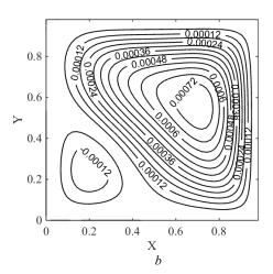
**Figure 9.** Contours of stream function with different heat flows on the left  $(q = 0.05 \text{ W/m}^2)$  and right  $(q = 0.05 \text{ W/m}^2)$  to boundary with: a) heat insulation on lower boundary (q = 0), b) with the heat flow on lower boundary  $(q = 0.05 \text{ W/m}^2)$ .
