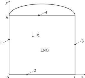
**Figure 1.** Solution area to the problem: 1 – the solution region: 1, 2, 3 – boundary "LNG – wall", 4 – the free surface.
