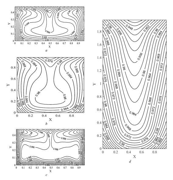
**Figure 3.** Fields temperature in the storage tanks LNG with different geometric dimensions: a)  $l = 10 \, \text{m}$ ,  $h = 5 \, \text{m}$ ; b)  $l = 10 \, \text{m}$ ,  $h = 10 \, \text{m}$ ; c)  $l = 10 \, \text{m}$ , h = 20; d)  $l = 20 \, \text{m}$ ,  $h = 10 \, \text{m}$ . The numerical values of coordinates and contour line of the function of current s are given in a dimensionless form.
