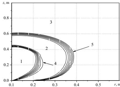
**Fig. 3.** Distribution of the volume fraction of coke upon heating the coal seam: 1 - an area in which the slag was; 2 - an area filled with char; 3 - unheated area filled with coal; 4 - boundary of coke oxidation; 5 - coal pyrolysis border.
