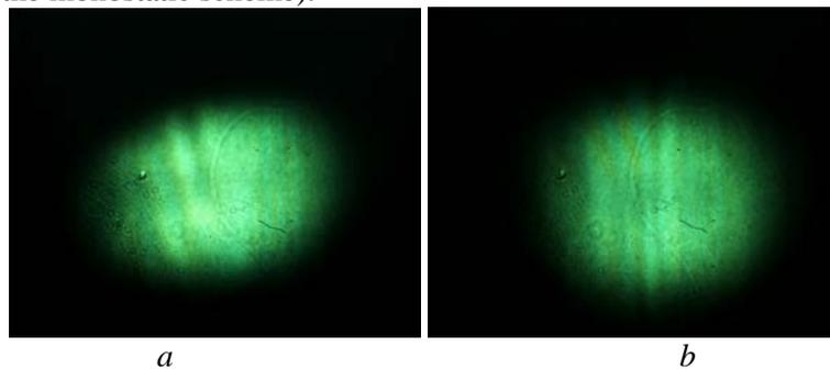
**Figure 3.** The photographs of laser beam profiles corresponding to: *a*) CuBr laser pulse duration of 170 ns, PRF of excitation of 2 kHz; *b*) CuBr laser pulse duration of 100 ns, PRF of excitation of 2.6 kHz. The heating temperature of the reservoir with CuBr powder is  $390^{\circ}\text{C}$ , voltage on the rectifier is 195 V, capacitance of storage capacitor is 4.95 nF.
