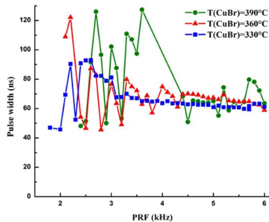
**Figure 4.** Influence of the PRF of excitation at various heating temperature of the reservoir with CuBr powder on the pulse duration of lasing. Voltage on the rectifier is 200 V, capacitance of storage capacitor is 1.65 nF.
