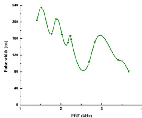
**Figure 2.** Influence of the PRF of excitation on the pulse duration of lasing. The heating temperature of the reservoir with CuBr powder is 390°C, voltage on the rectifier is 195 V, capacitance of storage capacitor is 4.95 nF.
