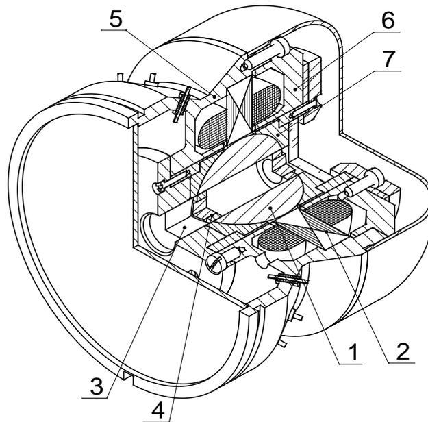
**Figure 1.** The construction of the gyroscope layout with a gas-dynamic suspension of ball rotor:
