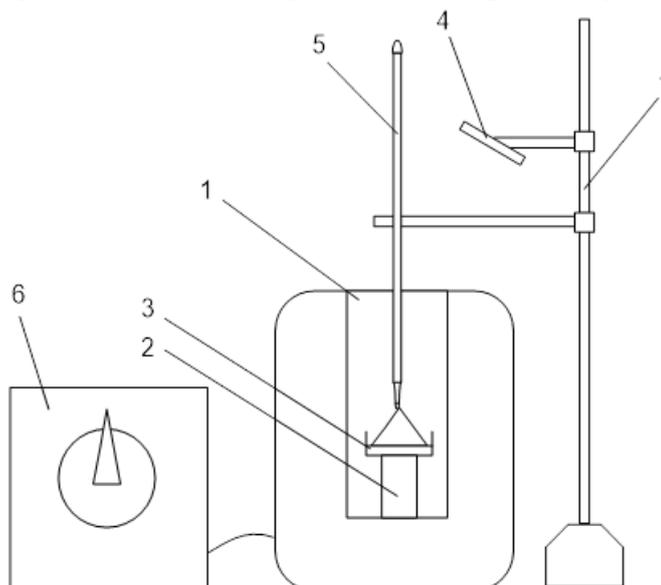
**Figure 1.** Circuitry of the instrument for determination of parameters of self-ignition of substances and materials: 1 – the electric furnace (V=1000ml); 2 – quartz support; 3 – a porcelain support for substance; 4 – viewing mirror; 5 – mercury thermometer; 6 – laboratory autotransformer; 7 – support.
