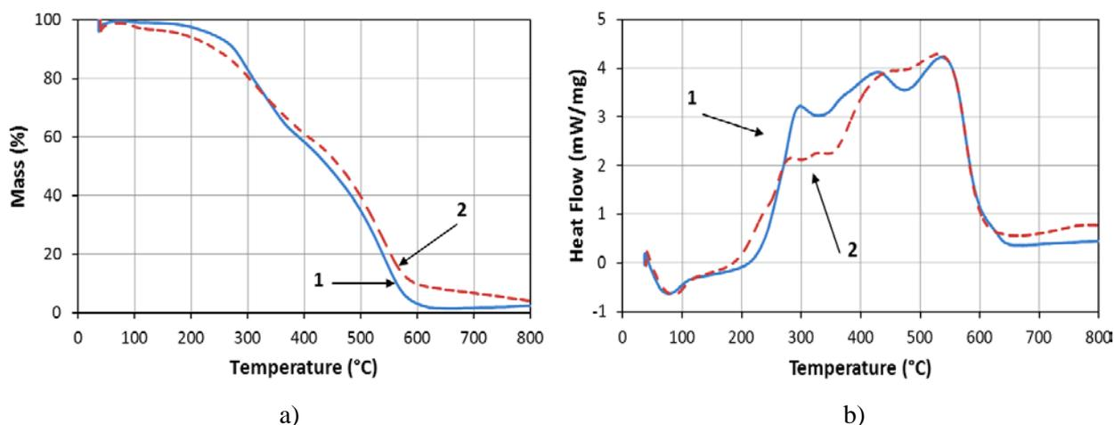
**Figure 2.** TG (a) and DSC (b) curves of the epoxy composites: 1 – unfilled epoxy polymer; 2 – epoxy polymer filled with 10 wt. % boric acid.
