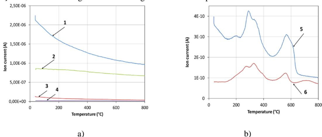
**Figure 1.** Dependence of ions current on temperature a)  $m/z = 28$  (1 and 2) and 44 (3 and 4); b)  $m/z = 30$  (5 and 6): 1, 3, 5 – unfilled epoxy polymer; 2, 4, 6 – epoxy polymer filled with 10 wt. % boric acid.
