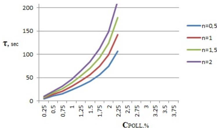
**Figure 2.** The rise time of the concentration of flammable vapors and gases in the volume of the mobile unit based on the ventilation rate.
