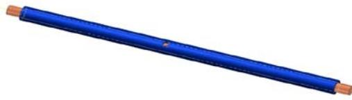
**Figure 3.** Example of a through defect.
