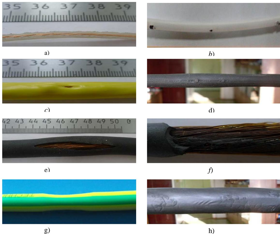
**Figure 1.** The main types of cable products insulation defects, insulation "slice" – a; impurity inclusion – b; local rupture of insulation and bumps – c, d, e; insulation material adhering on the cable cores – f, insulation porosity – g; outer diameter inequality, buildup along the insulation surface – h.
