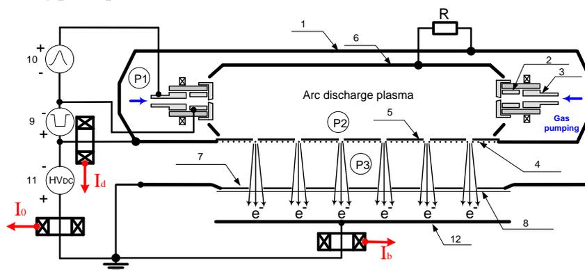
**Figure 1.** Schematic of a wide-aperture electron source: 1 – hollow anode, 2 – cathode, 3 – igniter electrode, 4 – emission grid, 5 – mask; 6 – screen 7 – support grid of extraction foil window, 8 – extraction foil, 9 - power supply of discharge, 10 – power supply of igniter, 11 – high voltage source, 12 – collector, P1, P2, and P3 – PMI-2 type manometric transducers.
