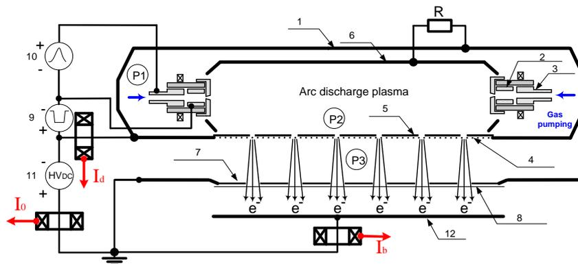
**Figure 1.** Schematic of a wide-aperture electron source: 1 – hollow anode, 2 – cathode, 3 – igniter electrode, 4 – emission grid, 5 – mask; 6 – screen 7 – support grid of extraction foil window, 8 – extraction foil, 9 - power supply of discharge, 10 – power supply of igniter, 11 – high voltage source, 12 – collector, P1, P2, and P3 – PMI-2 type manometric transducers.
