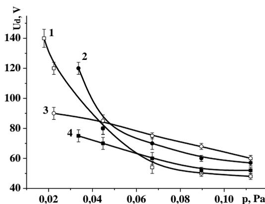
**Figure 8.** Arc discharge operating voltage  $U_d$  vs the pressure  $p$  at a discharge current of 150 (1,4) and 250 A (2,3) for the cathode assemblies with a constriction channel diameter of 6 (2,4) and 11 mm (1,3).
