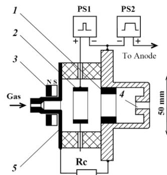
**Figure 3.** Cathode assembly with arc initiation by a reflex discharge. 1 – Mg cathode, 2 – anode, 3 – permanent magnet, 4 – constriction channel, 5 – auxiliary cathode. PS1 – auxiliary discharge power supply, PS2 – arc discharge power supply.
