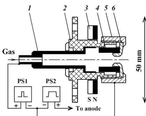
**Figure 1.** Cathode assembly: 1 – trigger electrode with gas supply, 2 – insulator, 3 – ring magnet, 4 – hollow magnesium cathode, 5 – stainless steel nut, 6 – ferromagnetic insert; PS1 – auxiliary discharge power supply, PS2 – arc discharge power supply.
