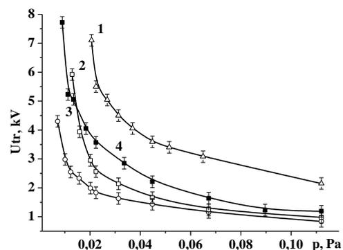
**Figure 4.** Auxiliary discharge initiating voltage  $U_{tr}$  vs the pressure  $p$  at a constriction channel diameter of 6 (1), 11 (2), 10 (3), and 11 mm (4); the width of the reflex discharge ring anode is increased from 6 to 23 mm.
