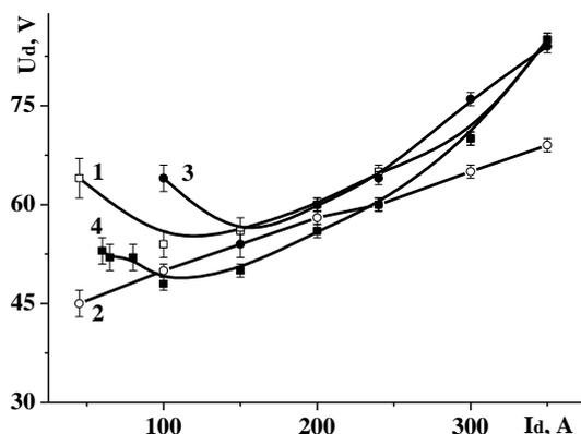
**Figure 7.** Current-voltage characteristics of the arc discharge for the cathode assemblies with a constriction channel diameter of 6 (1,2) and 11 mm (3,4) at  $p=0.067$  Pa (1,3) and  $p=0.11$  Pa (2,4).
