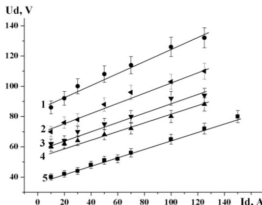
**Figure 2.** Current-voltage characteristics of arc discharges at  $p = 50$  mPa (Ar) for different cathode assemblies: 1 – cathode assembly based on a Penning cell [13]; 3,4 – cathode assembly based on an open arc with a tungsten and magnesium cathode, respectively [7]; 2,5 – new cathode assembly with no and with a ring magnet, respectively.
