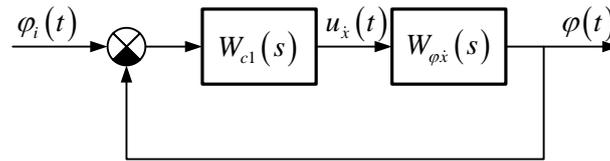
**Figure 6.** Control system block diagram of channel  $\varphi \rightarrow \dot{x}$
