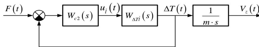
**Figure 8.** Control system block diagram of channel  $\Delta T \rightarrow \dot{l}$
