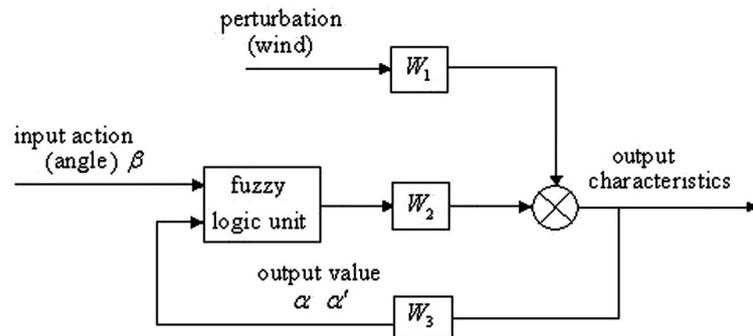
**Figure 2.** The block diagram of the modelled system.
