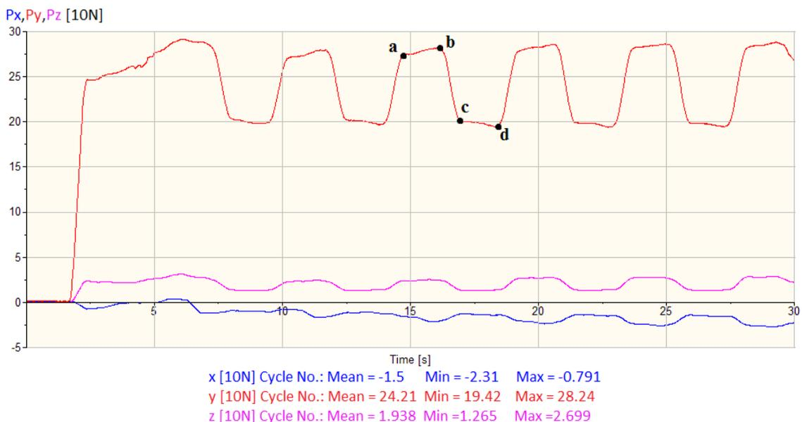
**Figure 4.** Relationship between burnishing force components  $P_y$ ,  $P_x$  and  $P_z$  (kN) and time  $T$  (s) during burnishing with a coil spring actuated tool. Burnishing parameters: radius of the indenter  $R_{sp}=2$  mm; feed rate  $S=0.05$  mm per rev.; burnishing speed  $v\approx 0.02$  m/s; angular velocity  $\omega=1.3$  s<sup>-1</sup>.  $\Delta P_y\approx 88$  N.
