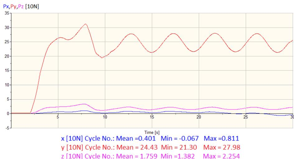
**Figure 2.** Relationship between burnishing force components  $P_y$ ,  $P_x$  and  $P_z$  (kN) and time  $T$  (s) during burnishing with a dynamometric tool with a flat spring. Burnishing parameters: radius of the indenter  $R_{sp}=2$  mm; feed rate  $S=0.05$  mm per rev.; burnishing speed  $v\approx 0.02$  m/s; angular velocity  $\omega=1.3$  s<sup>-1</sup>.  $\Delta P_y\approx 67$  N.
