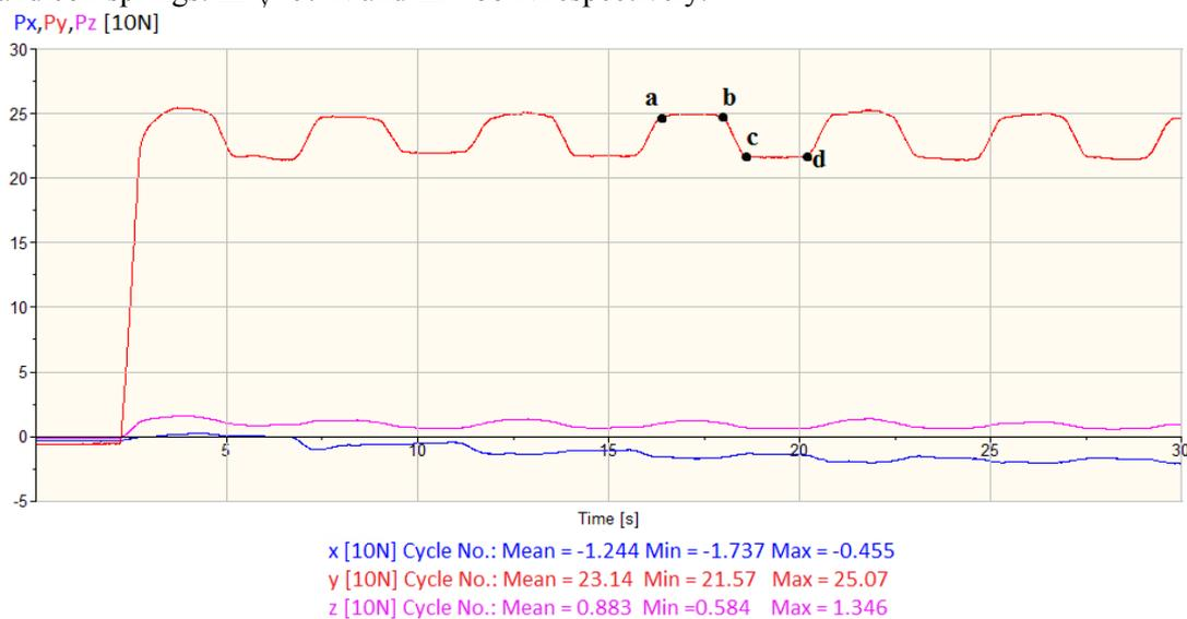
**Figure 7.** Relationship between burnishing force components  $P_y$ ,  $P_x$  and  $P_z$  (kN) and time  $T$  (s) during burnishing with a pneumatic tool equipped with a receiver (bellows with compressed air is an actuator). Burnishing parameters: radius of the indenter  $R_{sp}=2$  mm; feed rate  $S=0.05$  mm per rev.; burnishing speed  $v \approx 0.02$  m/s; angular velocity  $\omega=1.3$  s<sup>-1</sup>.  $\Delta P_y \approx 35$  N.
