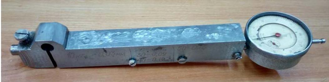
**Figure 1.** Dynamometric burnishing tool (an actuator is a flat spring with a vibration damper).
