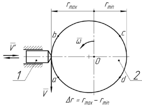
**Figure 5.** Movement of an indenter on the surface with radial run-out (eccentric surface). 1 – indenter; 2 – surface being burnished.  $V$  – burnishing speed, m/s;  $V'$  – sliding speed of an indenter with a plunger relative to the body of the burnisher;  $\omega$  – angular velocity of the workpiece,  $s^{-1}$ .
