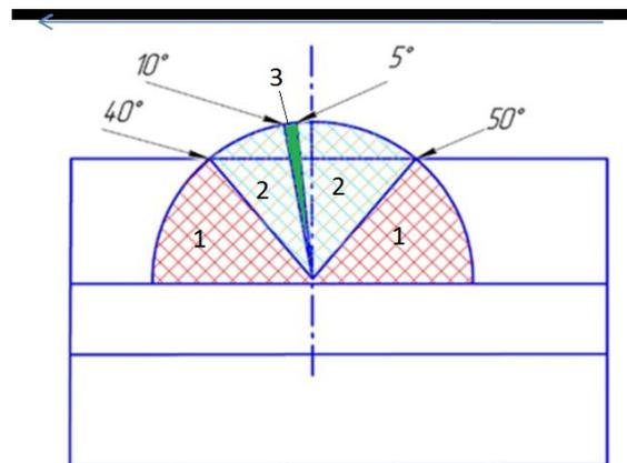
**Figure 4** Defectless formation zones according to incline angle of the torch along the weld axis (zone 1 – zone of incline angle of the torch providing no complete penetration; zone 2 – zone of higher splattering; zone 3 – zone with recommended incline angle of the torch)
