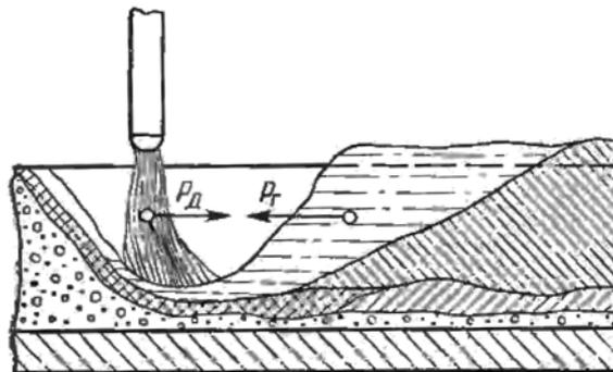
**Figure 3** Forces affecting the weld pool
