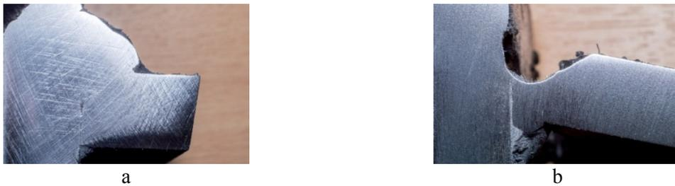
**Figure 2** Incomplete fusion without the gap (a), with big gap but insufficient current strength (b)
