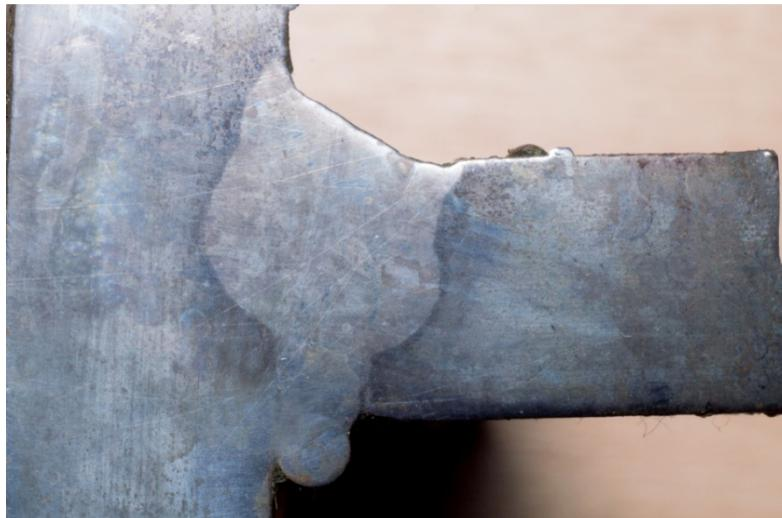
**Figure 8.** A metallographic section of a root weld of 12 mm T-joint
