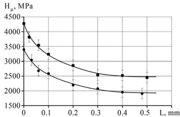
**Figure 3.** Depthward distribution of micro-hardness after ultrasonic treatment:
