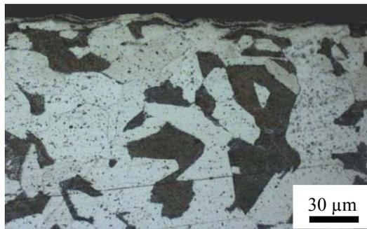
**Figure 2.** Metallography steel 20 after ultrasonic treatment
