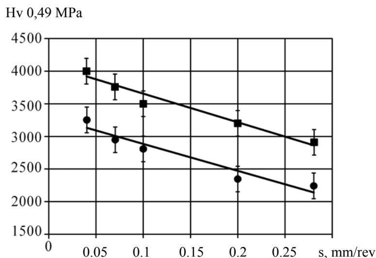
**Figure 11.** Effect of indenter feed on micro-hardness after ultrasonic treatment: ● - Steel 20; ■ - steel 40X. Processing velocity 23 m/min
