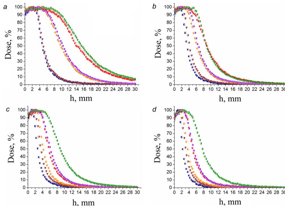
**Figure 2.** The electron beam depth dose distribution in the test materials with density: a – 1.1 g/cm<sup>3</sup>; b – 1.5 g/cm<sup>3</sup>; c – 2.0 g/cm<sup>3</sup>; d – 2.5 g/cm<sup>3</sup>.
