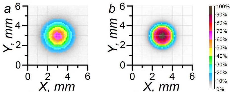
**Figure 5.** The electron beam shape in the transverse plane at the depth 3.67 mm in the ABS-plastic modified by a – lead and b – zinc (the test material density – 2.0 g/cm<sup>3</sup>; the electron beam energy – 12 MeV).
