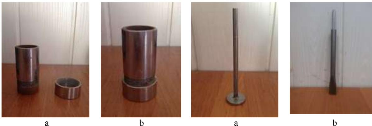
**Figure 1.** A metal cartridge for elastomer's samples testing: a – in the disassembled condition; b– in the assembled condition.
