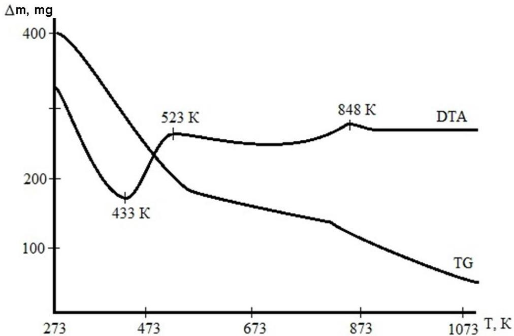
**Figure 3.** Thermogram of the  $\text{SiO}_2 - \text{P}_2\text{O}_5$  formation by decomposing FFS based on tetraethoxysilane and orthophosphoric acids
