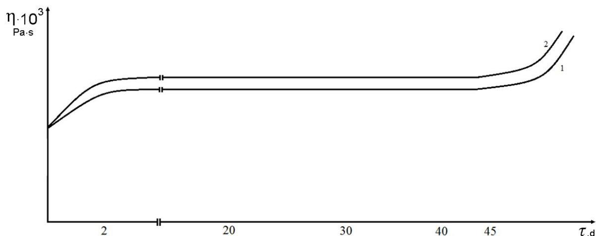
**Figure 2.** Time-dependent changes in viscosity of the FFSs with boric acid added: 1  $B_2O_3$ - 10% by wt.; 2  $B_2O_3$ - 30% by wt.
