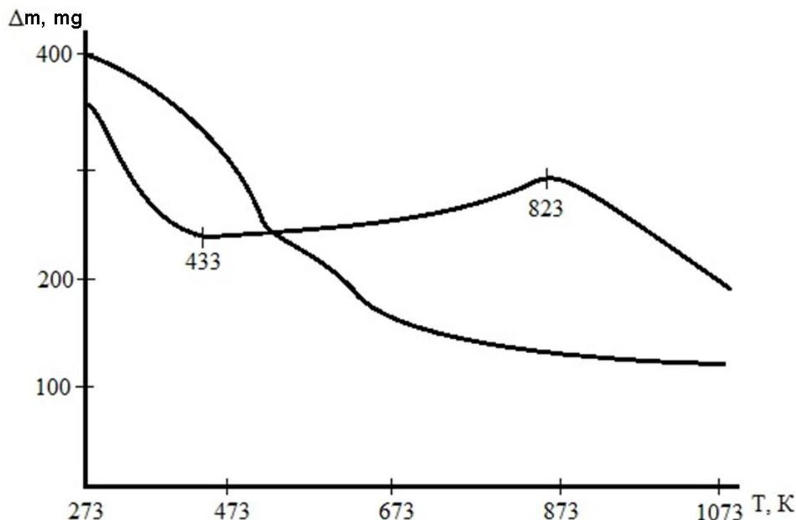
**Figure 4.** Thermogram of the  $\text{SiO}_2 - \text{B}_2\text{O}_3$  formation by decomposing FFS based on tetraethoxysilane and boric acid
