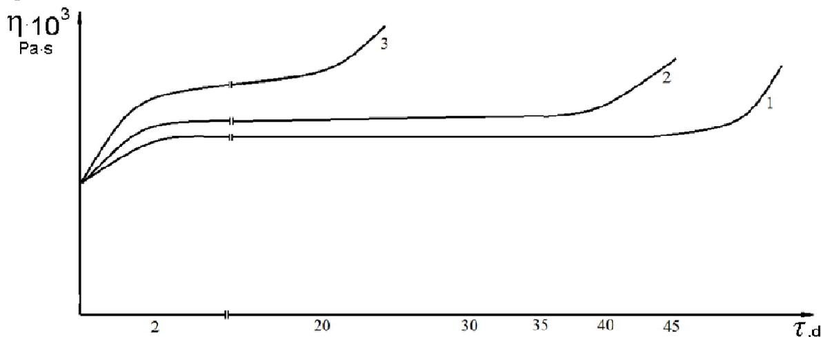
**Figure 1.** Time – dependent changes in viscosity of the FFSs with orthophosphoric acid added: 1  $\text{P}_2\text{O}_5$  – 10% by wt.; 2  $\text{P}_2\text{O}_5$  – 20% by wt.; 3  $\text{P}_2\text{O}_5$  – 30% by wt.
