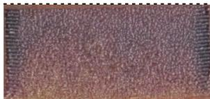
**Figure 4.** Micrographs, showing surfaces of the sintered copper samples (x2), process conditions of sintering:  $V=3000$  mm/min,  $t=200$  °C,  $S=0.3$  mm,  $P=15$  W.
