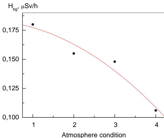
**Figure 3.** Background radiation value dependence from the weather type, spring: 1 - clear weather, 2 - cloudy weather, 3 - overcast weather;  $H_{bg}$  – background dose rate of gamma-radiation.
