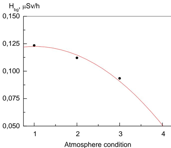
**Figure 4.** Background radiation value dependence from the weather type, autumn: 1 - clear weather, 2 - cloudy weather, 3 - overcast weather;  $H_{bg}$  – background dose rate of gamma-radiation.
