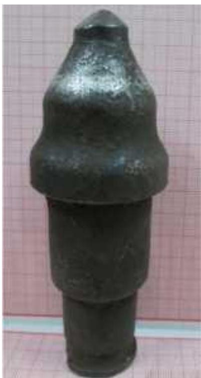
Figure 3. Early wear of a pick body around the tip
