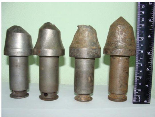
Figure 1. Picks wear over time
