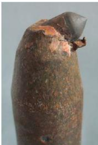
Figure 2. RKS-1 pick with a hard-alloy insert broken out
