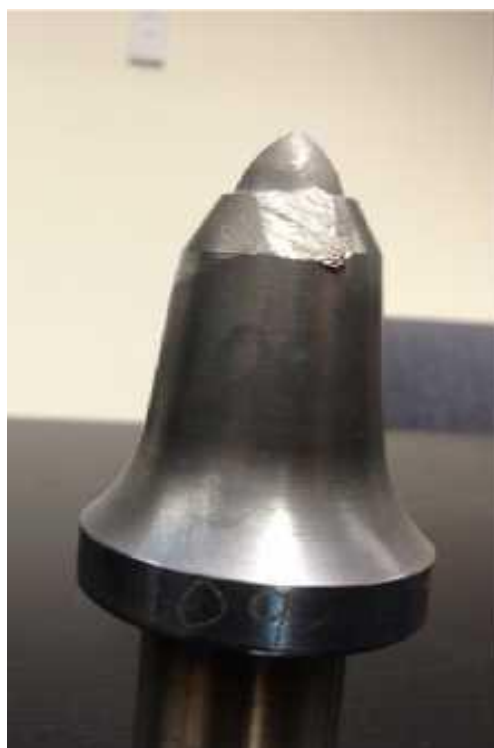
Figure 3. Early wear of a pick body around the tip
