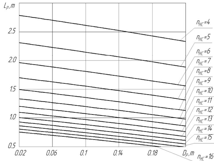
Figure 2. Dependence of the safe distance by stability condition
