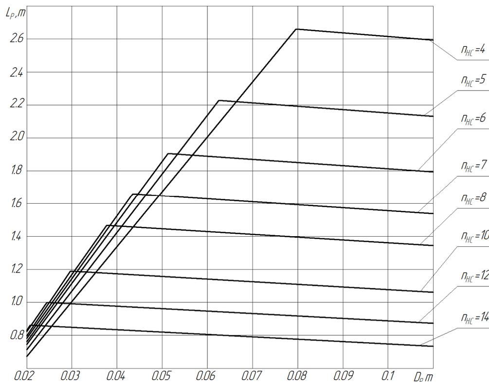
Figure 4. Dependence of safe distance by design arrangement condition and stability condition
