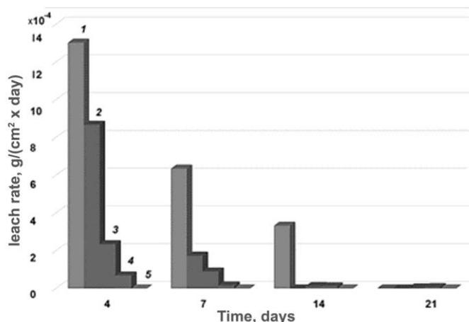
**Figure 1.** Radionuclide leach rates from the zirconium alloy: 1 –  $^{90}\text{Sr}$ ; 2 – actinides; 3 –  $^{137}\text{Cs}$ ; 4 –  $^{60}\text{Co}$ ; 5 –  $^{94}\text{Nb}$ .
