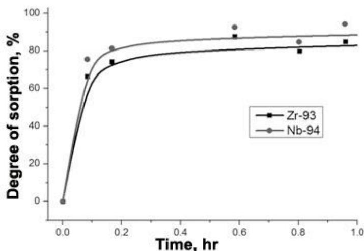
**Figure 2.** The sorption kinetics of  $^{93}\text{Zr}$  and  $^{94}\text{Nb}$  radionuclides on the barrier material.
