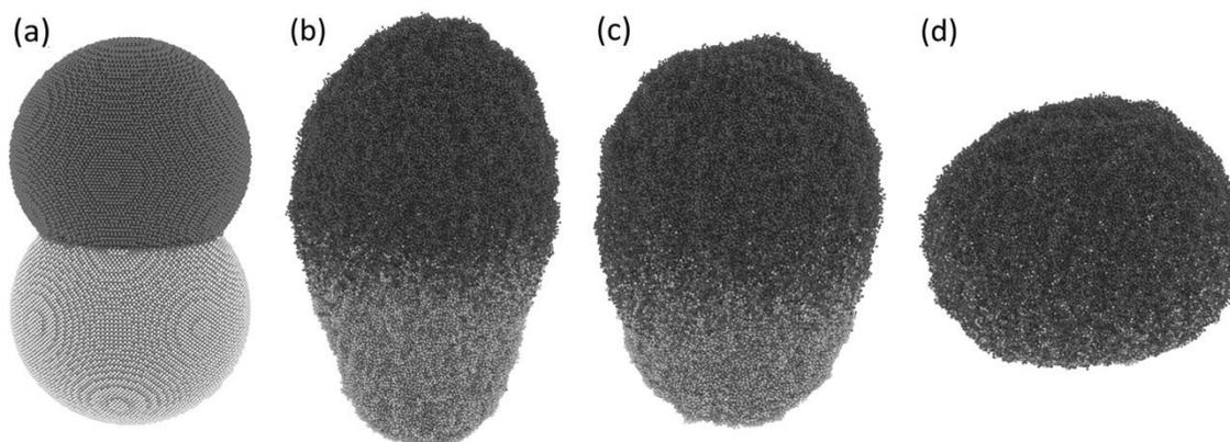
**Figure 1.** (a) The initial structure of the modeled particles of Ti (dark gray) and Nb (light gray) and structure corresponds to different moments of time of the high-speed heating process up to 6000K: (b) 70 ps, (c) 120 ps and (d) 220 ps.
