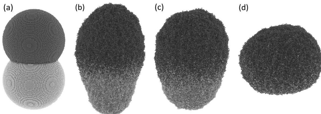
**Figure 1.** (a) The initial structure of the modeled particles of Ti (dark gray) and Nb (light gray) and structure corresponds to different moments of time of the high-speed heating process up to 6000K: (b) 70 ps, (c) 120 ps and (d) 220 ps.
