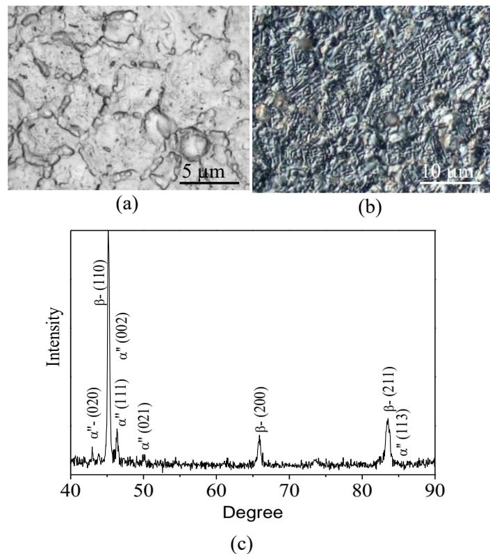
**Figure 3.** Optical images of the microstructure (a, b) and X-ray diffractogram fragment of the sample (c)
