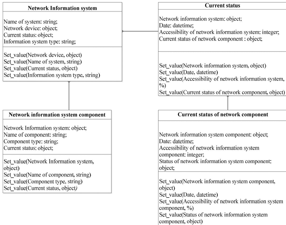
Figure 3. A fragment of the components model of network infrastructure monitoring system
