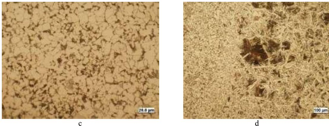
**Fig. 3** – Weld microstructure: a,b – microstructure of 09G2S steel, c – microstructure of welded joint heat affected zone (low frequency modulation current welding); d – microstructure of welded joint heat affected zone (conventional feed of welding wire)
