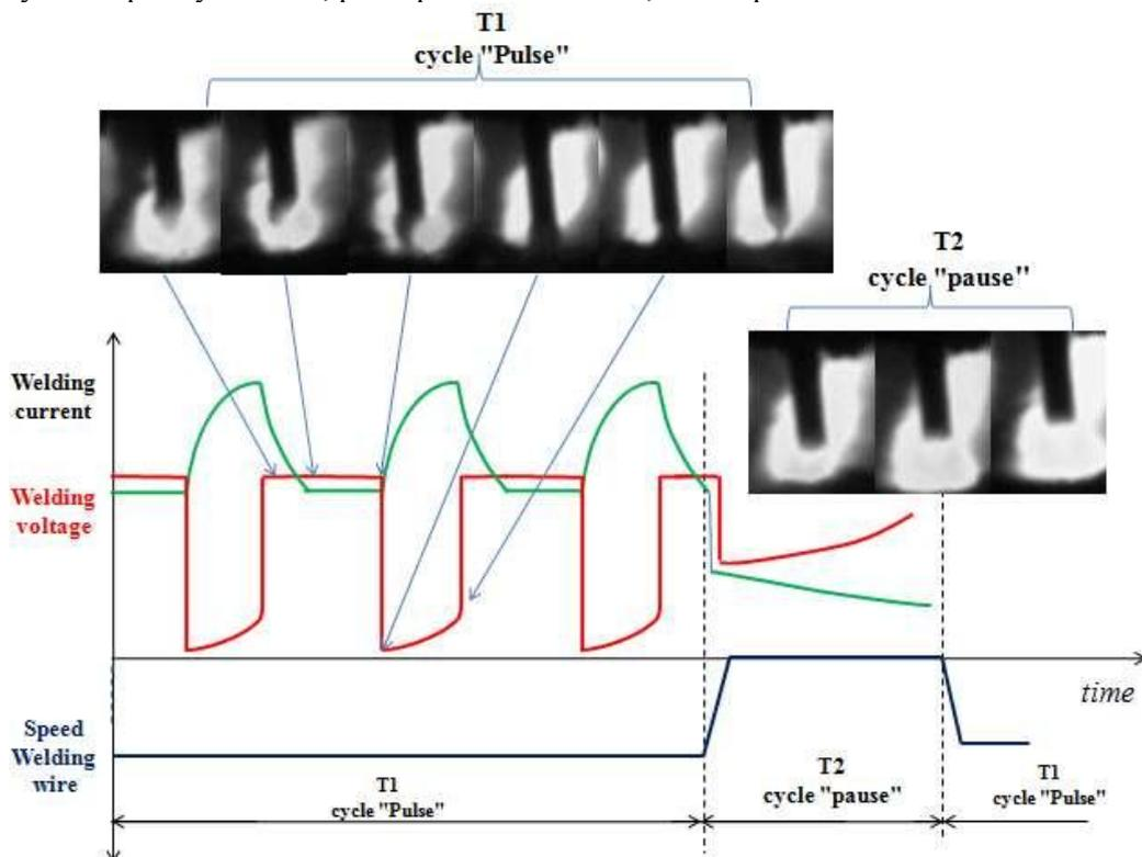
Fig.1 Welding cyclogram
