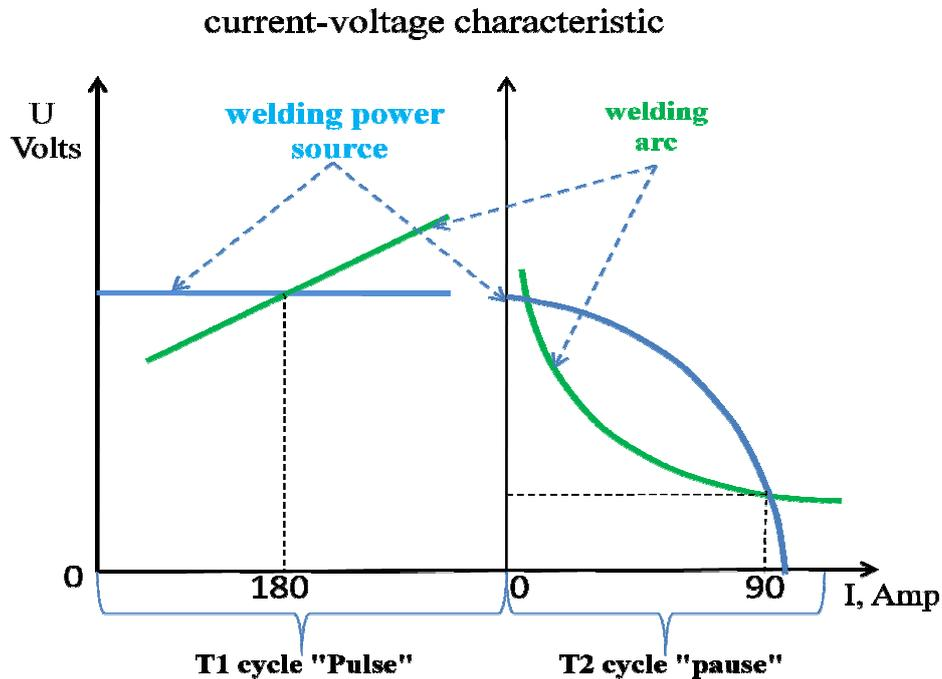
**Fig 2.** Interdependence of current-voltage characteristic of the arc and of the power supply at different intervals of welding process.
