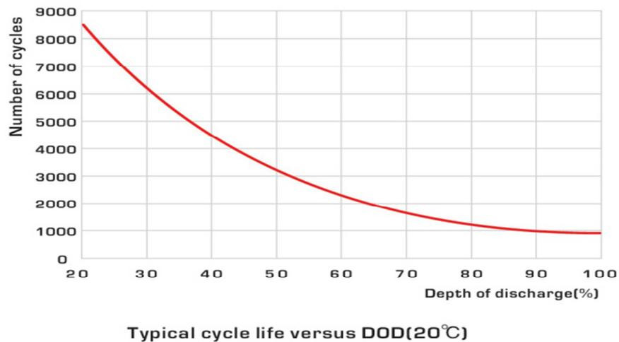
Figure 7- Depth of discharge nickel- iron battery [9]
