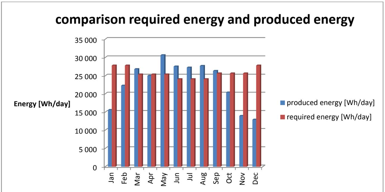
*Figure 16- Comparison required energy and produced energy*
