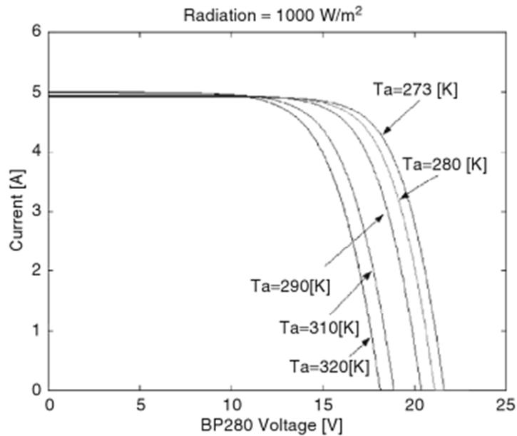
Figure 2- Effects of temperature on silicon solar cells [3]
