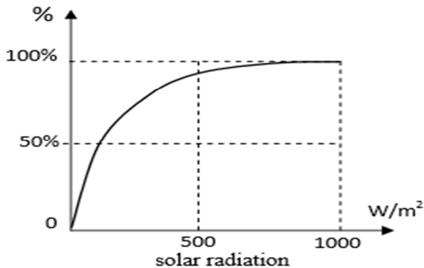
Figure 3- Efficiency dependence of photoconversion on solar radiation [6]
