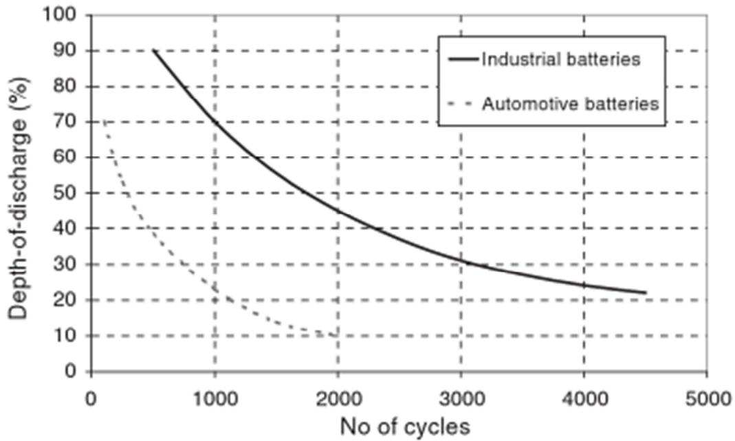
Figure 5- Nominal number of battery cycles vs depth of discharge [3]
