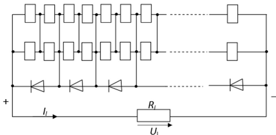
Figure 4- Bypass diodes connection circuit
