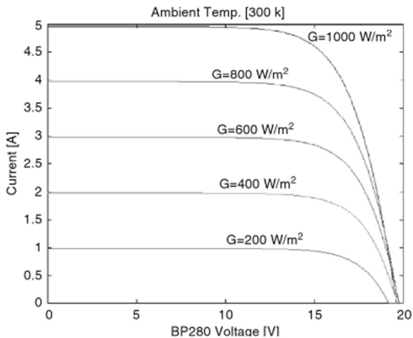
Figure 1- Typical current/ voltage characteristic curves for different insolation
