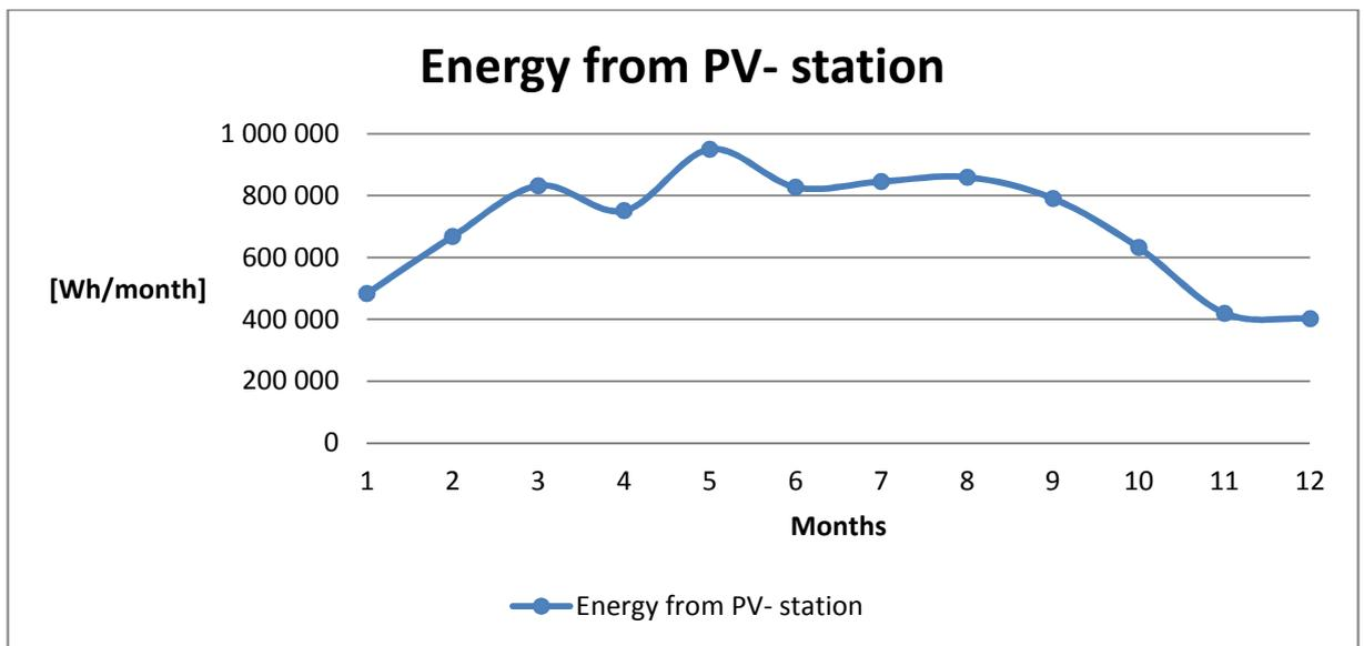
Figure 15- Energy from PV-station
