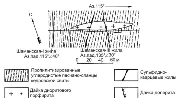
**Fig. 2.** Crossing of diorite porphyrite dyke of the Kedrovskiy golden-ore deposit by the sulfide-quartz Shamanskaya-III vein and dolerite dyke (plan). Left column (top to bottom): 1) Proptized carbonic sand-shales of the Kedrovskiy series; 2) Diorite porphyrite dyke. Right column (top to bottom): 1) Sulfide-quartz veins; 2) Dolerite dyke
