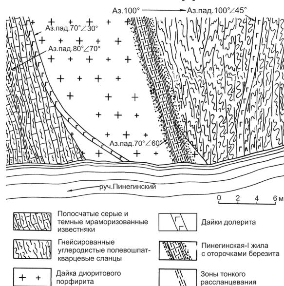
**Fig. 1.** Crossing of diorite porphyrite dyke of the Kedrovskiy golden-ore deposit by dolerite dyke and the sulfide-quartz Pineginskaya-I vein (plan). Left column (top to bottom): 1) Striate grey and dark marbled limestones; 2) Gneised carbonic feldspar-quartz shales; 3) Diorite porphyrite dyke. Right column (top to bottom): 1) Dolerite dyke; 2) The Pineginskaya-I vein with beresite frame; 3) Zones of thin shale
