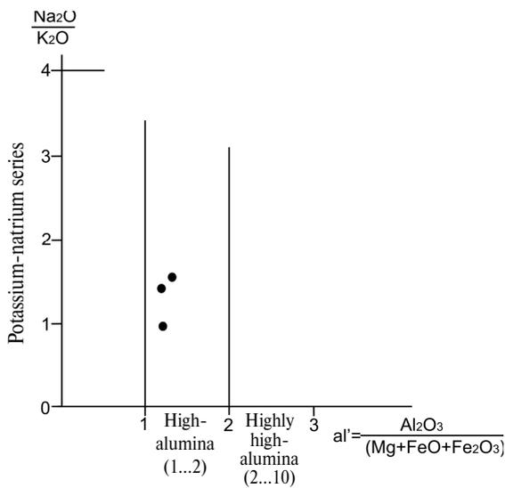
**Fig. 4.** Position of dykes' average structured magmatic rocks of the Kedrovskiy golden-ore in coordinates  $Na_2O/K_2O - Al_2O_3/(MgO+FeO+Fe_2O_3)$
