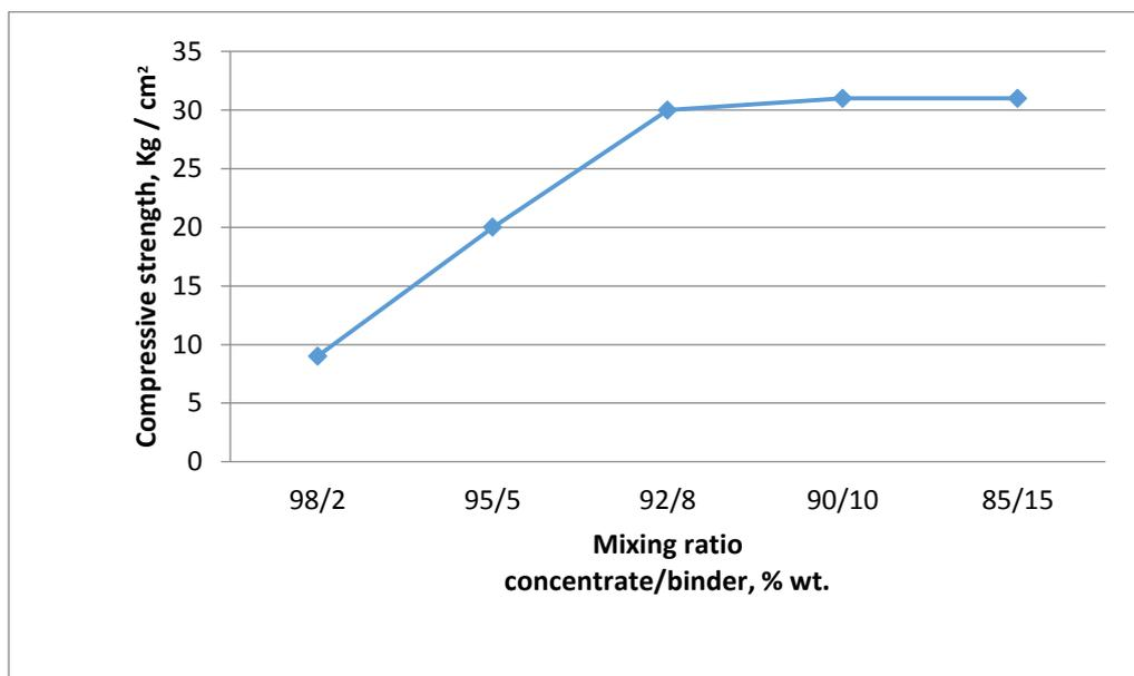
**Figure 2.** Dependence of briquette strength on the binder content
