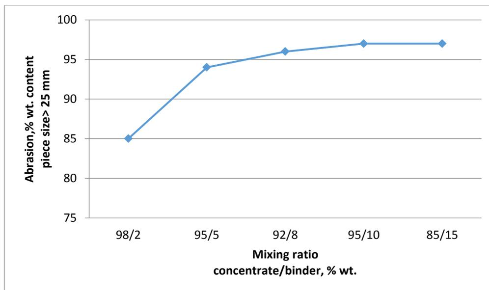
**Figure 3.** Dependence of briquettes abrasion on the content of binder
