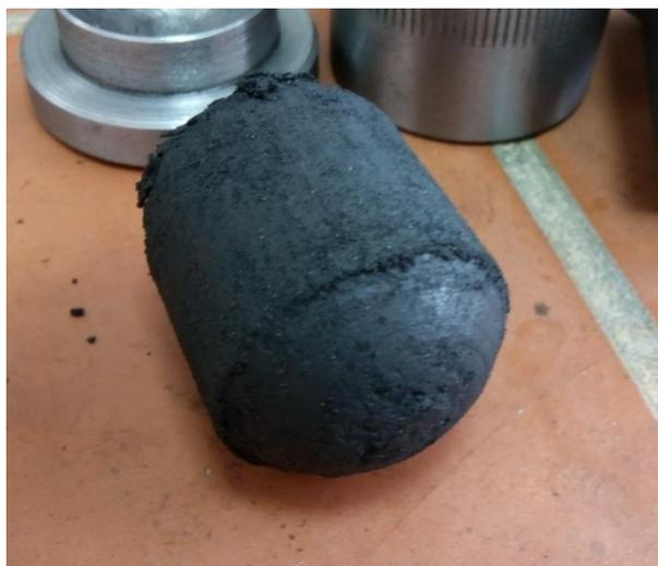
**Figure 1.** Briquetted fuel sample
