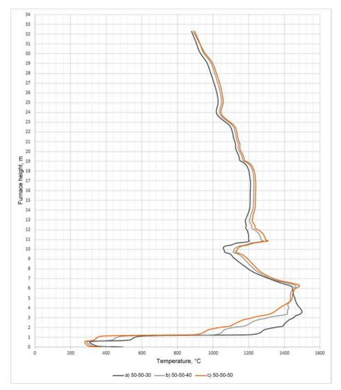
Fig. 3. Mean value of temperature through furnace height.
