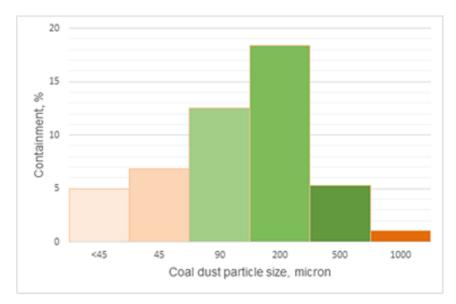
Fig. 2. Coal dust size analysis results.
