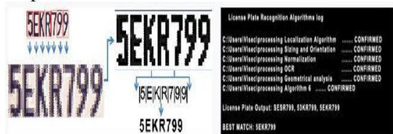
Figure 10 – Final stage after realization
