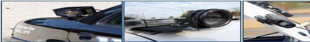
Figure 1 – Examples of Trunk and Lightbar Mounted Mobile LPR Cameras
