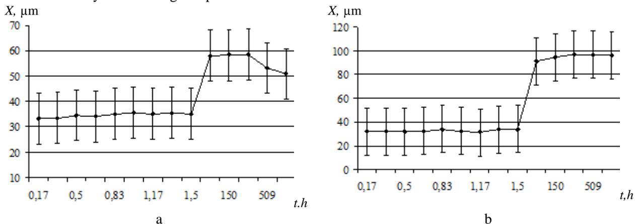
**Figure 5.** Dependence of calcium oxalate monohydrate particle sizes on the crystallization time in the presence of seeds: a) calcium oxalate; b) hydroxyapatite.
