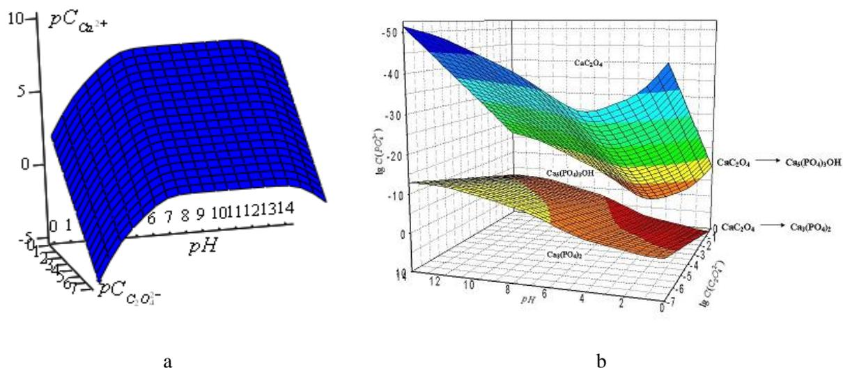
**Figure 6.** Stability fields observed during formation of poorly soluble compounds from the saline solution at 37°C and ionic strength of 0.3 M for the systems: a)  $\text{Ca}^{2+}-\text{C}_2\text{O}_4^{2-}-\text{H}_2\text{O}$ ; b)  $\text{Ca}^{2+}-\text{C}_2\text{O}_4^{2-}-\text{PO}_4^{3-}-\text{H}_2\text{O}$ .
