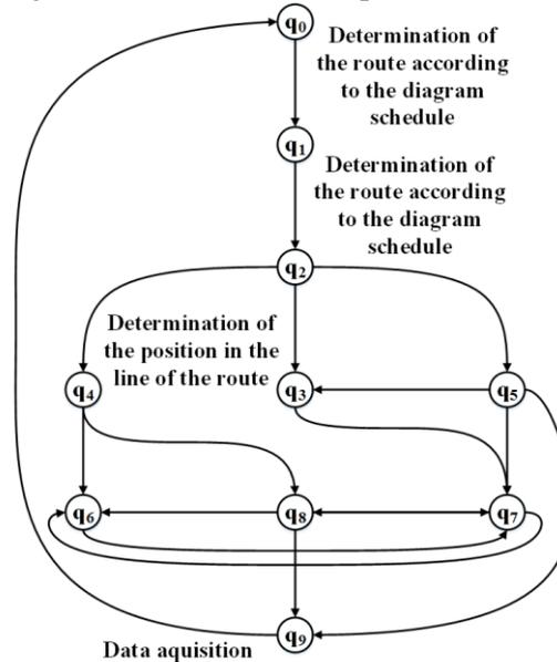
**Figure 3.** The scheme of the finite-state machine
