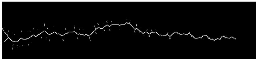
**Figure 3.** The crack skeleton.
