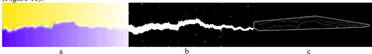
**Figure 1.** Crack detection by the analysis of the image series based on object motion data: (a) the optical flow pattern; (b) differentiation of the optical flow; (c) selecting the region of probable crack location
