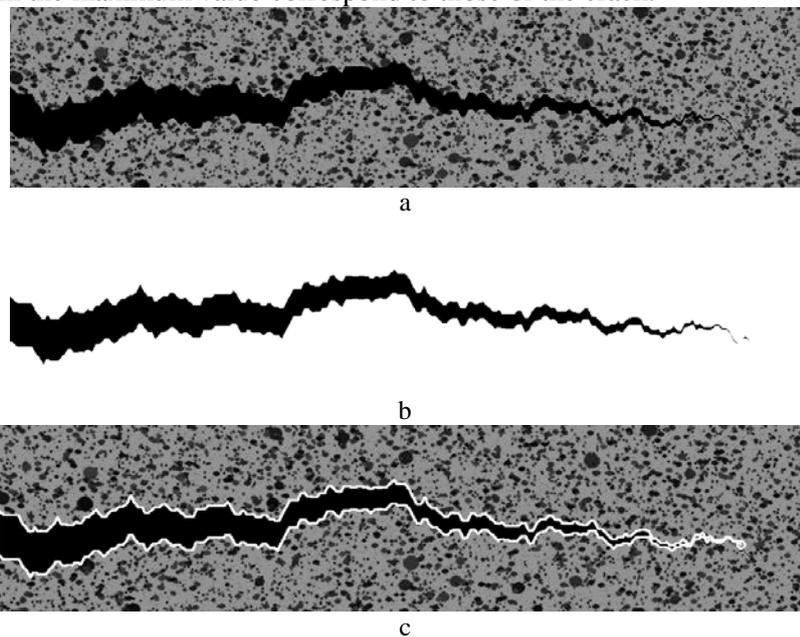
**Figure 2.** Crack detection by the analysis of individual images based on the contour detection: (a) input image; (b) binarized image used for segmentation; (c) detected crack
