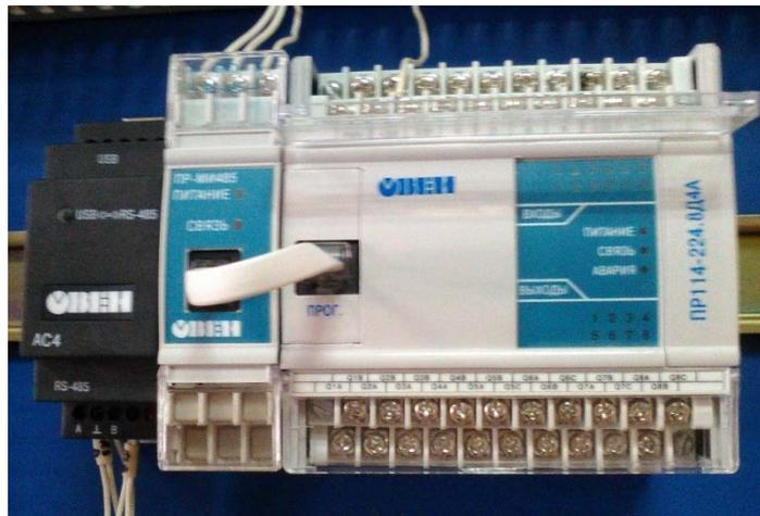
Figure 2. Programmable Relay PR114 OWEN
