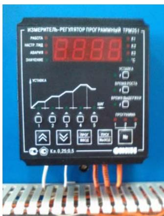
Figure 1. Program PID controller OWEN TRM251
