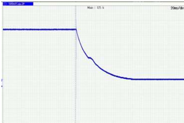
Figure 5. The oscillogram of the current in the load at closing thyristor VS.
