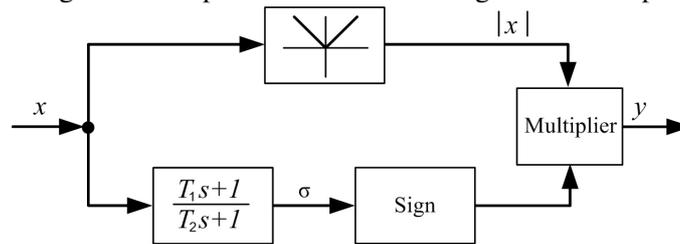
**Figure 2.** The pseudo-linear correcting device with phase advance
