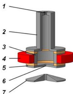
**Figure 3.** The electrode system of plasma cathode gun: 1 – the gas flow channel, 2 - the hollow cathode, 3 - the anode, 4 - the permanent magnet, 5 - the emitter cathode; 6 - the emission channel, 7 - the extractor (accelerating electrode) [2].
