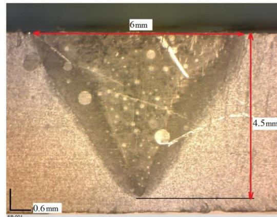
**Figure 7.** The macrostructure of the molten zone at  $t = 0.65 \text{ s}$ .
