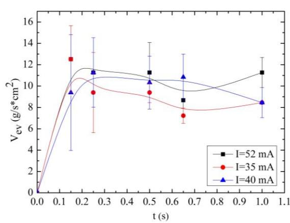
**Figure 5.** The dependence of the evaporation rate on the electron beam pulse duration.
