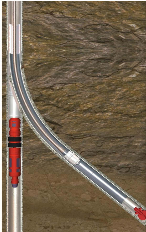
Figure 3 – A combination of SET technology and multilateral window milling systems can result in slimmer wells, reduced CAPEX and minimal environmental impact.
